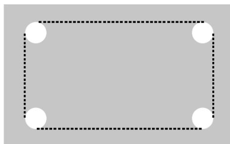
When making rectangular spaces inside the plate, we shall previously drill out holes on the rectangle's four corners, thus observing the recommended radii, and then making straight cuts joining the four drills.
